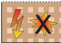
The components which could ignite a potentially explosive atmosphere are encapsulated in a casting compound. Thus once again the source of ignition and the potentially explosive atmosphere are kept separated.
