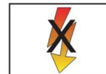
The production of sparks, arcs or excessive temperatures which might act as a source of ignition are prevented by additional measures and an increased degree of safety.
